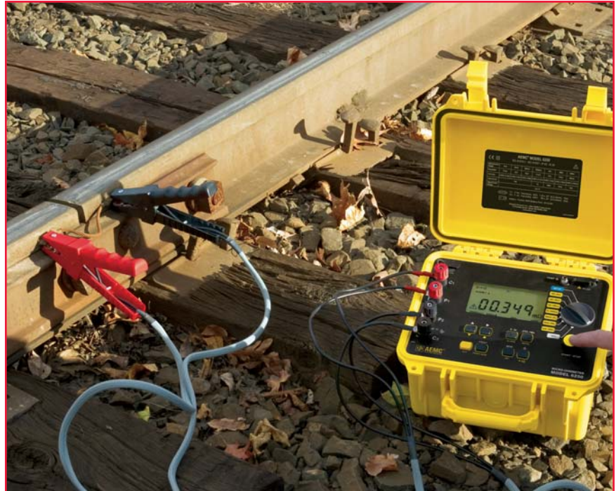
Verifying rail bonds with the Model 6250
