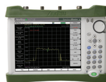
Spectrum Master Family MS2712E & MS2713E Compact Handheld Spectrum Analyzer
